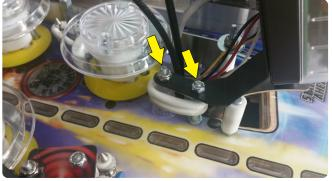
Remove 2 nuts holding Smartphone. (x1 5/16, x1 11/32).
