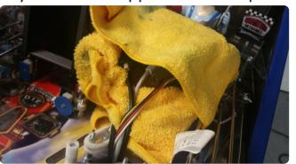
Wrap Smartphone assembly in soft cloth. Move aside to a safe place.
