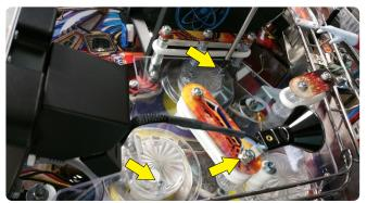
Turn off game. Remove Spotlight, then remove two screws that attach upper Playfield. Move upper PF to safe place.
