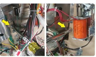
Lift playfield up. Remove both posts using 3/8" Driver and 3/8" Open End Wrench on front.
